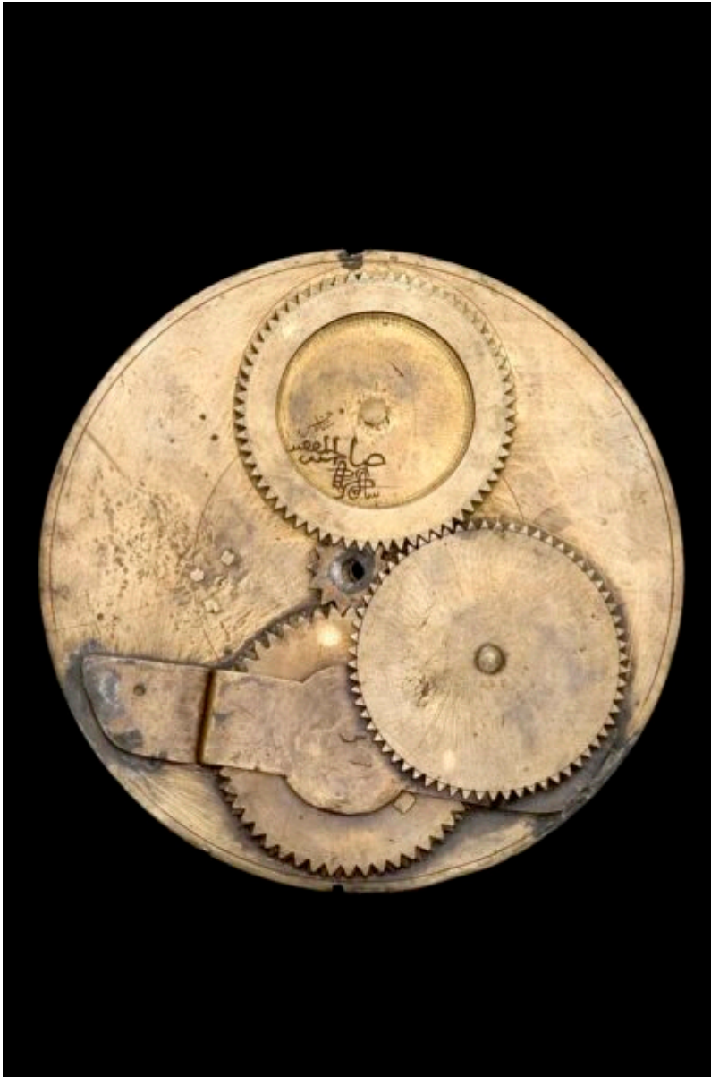
Muhammad b. Abi Bakr (Iranian, active 1200s), Astrolabe With a Geared Calendar (front and rear views) , 1221 or 1222, copper alloy, silvered copper alloy, silver, and wax; History of Science Museum, University of Oxford, images © History of Science Museum, University of Oxford.
